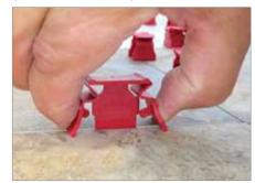
SeamClip works by interlocking the tiles, creating a single flat-slab surface while the setting material is curing. The interlocking design reduces or eliminates settling from shrinkage, and minimizes the possibility of warping. The result is a lippage-free mirror surface that reduces the need to re-lift tiles to add more mud, or to shim tiles.
